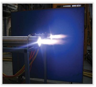
Plasma is an ionized, conductive gas at a temperature till 5 000 °C, which arises when a stream of the carrier gas (air enriched with 93 % oxygen) is passed through an arc discharge.
