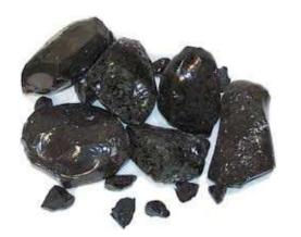
Plasma power=1000 Kwh/ton Volume reduction : 11:1
